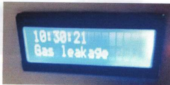
Figure 5.8: (a) Notification in mobile. (b) Warning in the LCD display.
