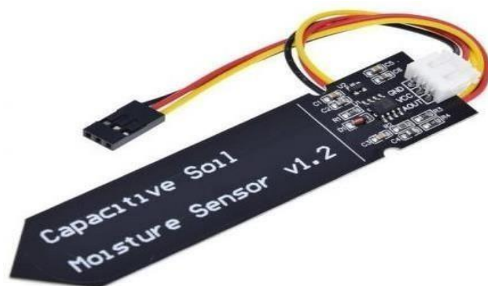
Figure 3.2. Capacitive Soil Moisture Sensor V1.2 [26]
