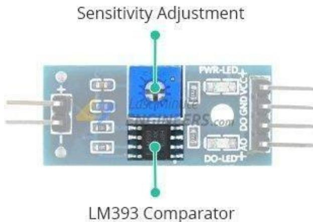
The module includes a potentiometer for adjusting the sensitivity of the digital output (DO).
