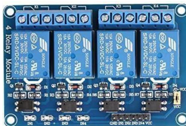
Figure 32. 4 Channel 5V Relay Module.
